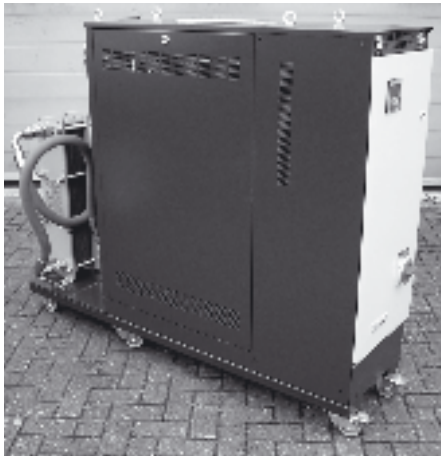
Figure 2: Temperature control unit with heat exchanger
