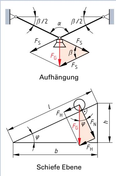
$$\beta = 180^\circ - \alpha \quad \Rightarrow \quad \alpha = 180^\circ - \beta$$
