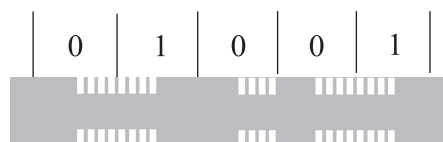
Figure F.4 - Manchester Biphase encoding
